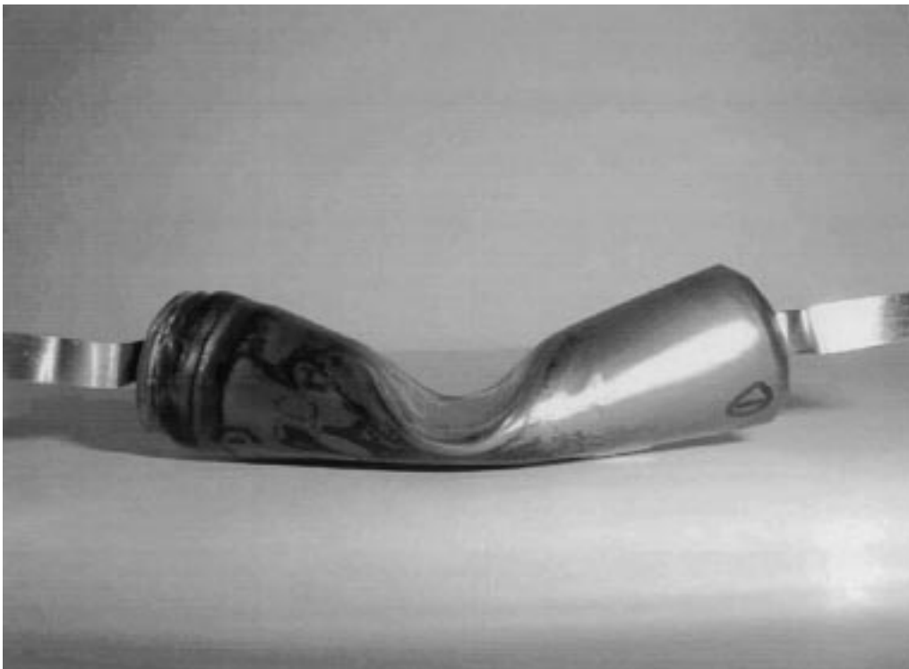
Fig. 3. Cell after crush test, stored for 1 month at 4.2 V and 60 °C.
